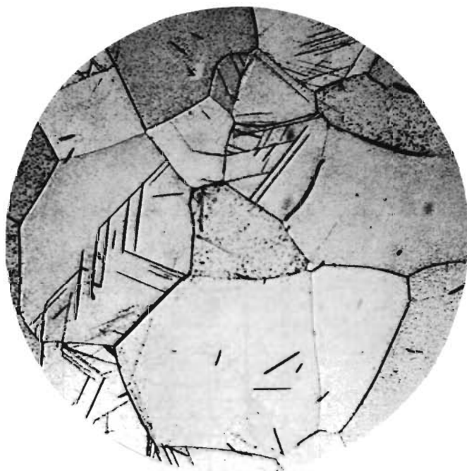
Fig. 3—Ti-22.2 pct Zr alloy; 675°C, 1464 hr; ice-brine-quenched; "A" etch, 10 sec; equiaxed \alpha ; X375. Enlarged approximately 28 pct for reproduction.
