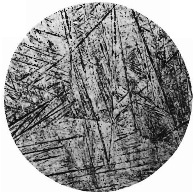
Fig. 9—Ti-50 pct Zr alloy; 525°C, 3048 hr; ice-brine-quenched; 675°C, 48 hr; ice-brine-quenched; "A" etch, 15 sec; transformed \beta ; X250. Enlarged approximately 28 pct for reproduction.
