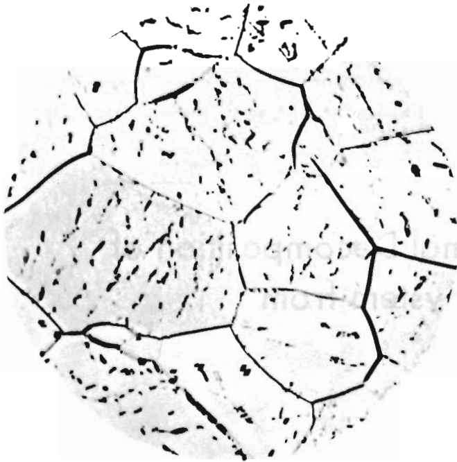
Fig. 6—Ti-29.0 pct Zr alloy; 600°C, 2616 hr; ice-brine-quenched; "R" etch, 15 sec; equiaxed \alpha ; X600. Enlarged approximately 28 pct for reproduction.
