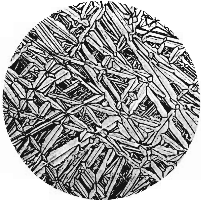
Fig. 8—Ti-50 pct Zr alloy; 525°C, 3048 hr; ice-brine-quenched; "R" etch, 5 sec; unrecrystallized \alpha ; X250. Enlarged approximately 28 pct for reproduction.
