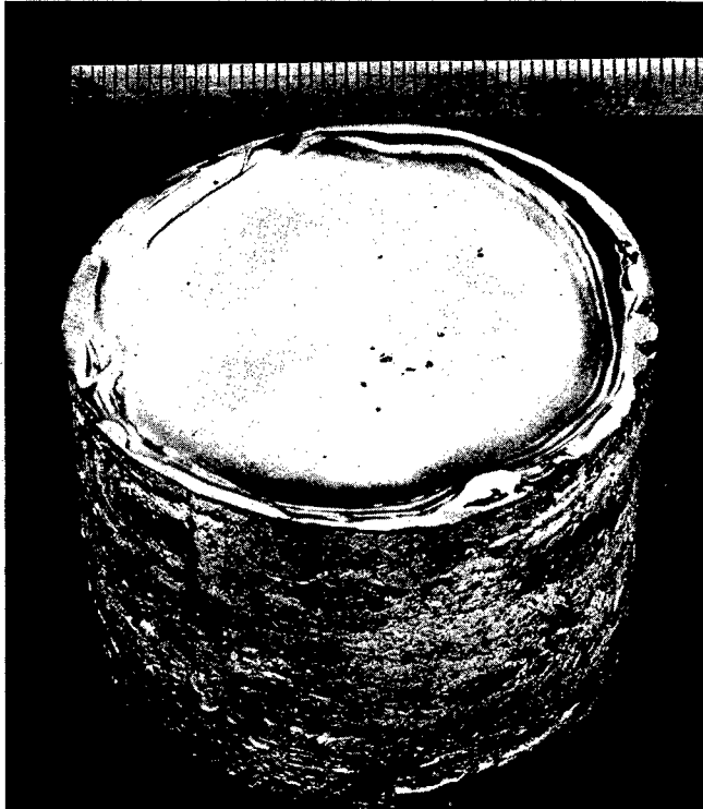
Figure 9. A 19-pound titanium ingot melted in a six-inch-diameter arc furnace. Surface roughness though not deep is ground off before the ingots are forged.
