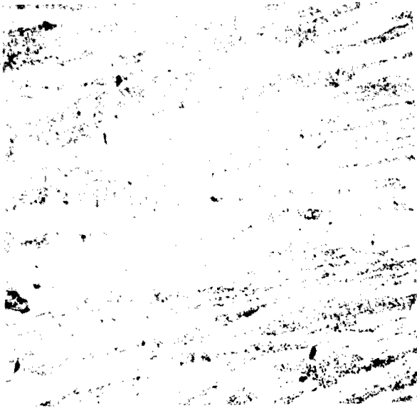
Fig. 22 X250 Alpha-Gamma Structure in 1.7% Ni Alloy Water Quenched after Hot Rolling and Soaking at 750° C.
