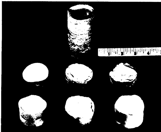
Figure 8. Small ingots of various refractory alloys melted in an arc furnace of an early design.
