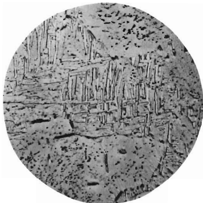
Fig. 7—Ti-39.6 pct Zr alloy; 600°C, 2616 hr; ice-brine-quenched; "R" etch, 15 sec; partially recrystallized \alpha + \beta ; X600. Enlarged approximately 28 pct for reproduction.
